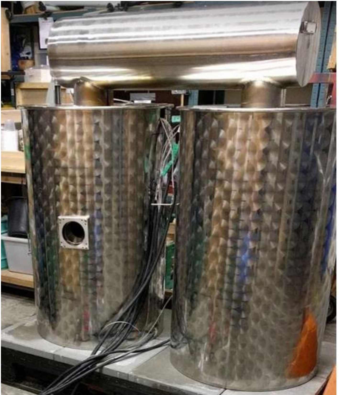
The Copenhagen Atomics Molten Salt experimental loop
